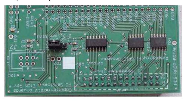
Here is a detailed view of the prototype area; there are tracks connecting the holes on the board in groups for easier layout. Note that
